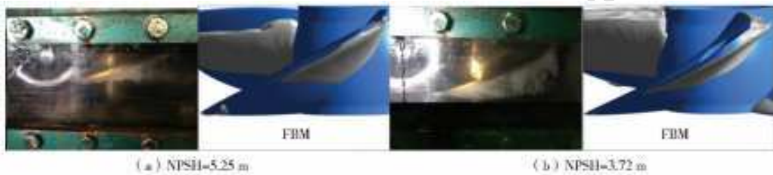
Fig. 5 Experimental and numerical calculation of cavitation distribution diagram
