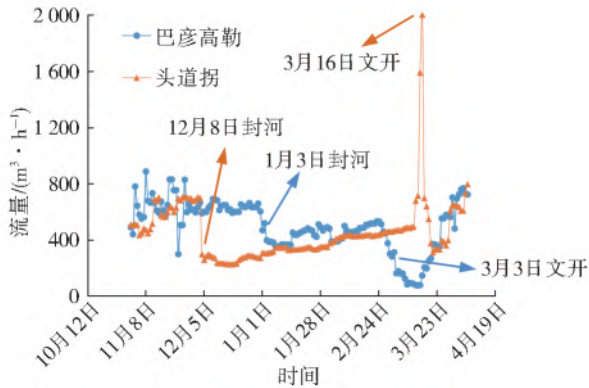
图2 2017—2018年巴彦高勒、头道拐日均流量变化曲线 Fig. 2 Average daily discharge change curve in Bayangaole and Toudaoguai from 2017 to 2018
