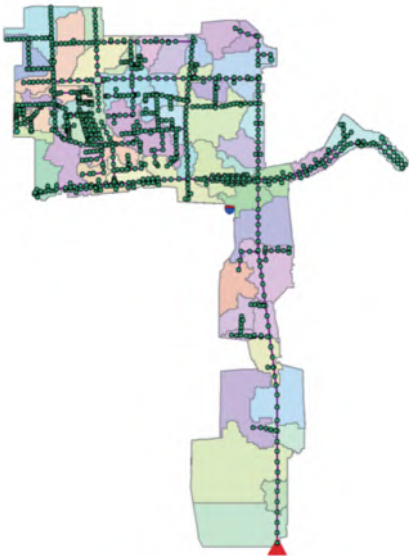
图 14 基于盆域分析划分的初级子汇水区 Fig. 14 The primary subcatchment based on basin analysis
