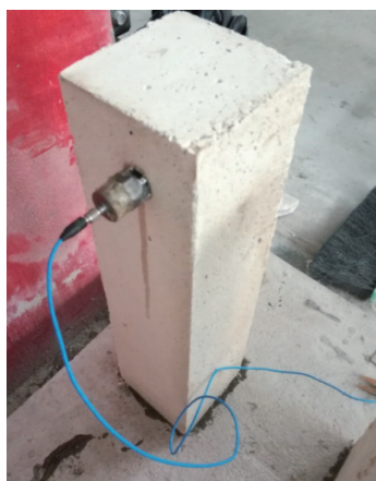
图 2 仿真混凝土材料动态弹性模量的测定 Fig. 2 The measurement of dynamic elastic modulus of emulation concrete material
