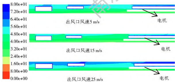
图 5 不同风速下隧洞空气温度分布云图(左端为掌子面) Fig. 5 Distribution of air temperature in the tunnel at different wind speeds (the tunnel face at the left end)
