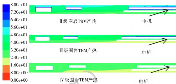
图 3 不同产热量下隧洞空气温度分布云图(左端为掌子面) Fig. 3 Distribution of air temperature in the tunnel under different heat production quantities (the tunnel face at the left end)
