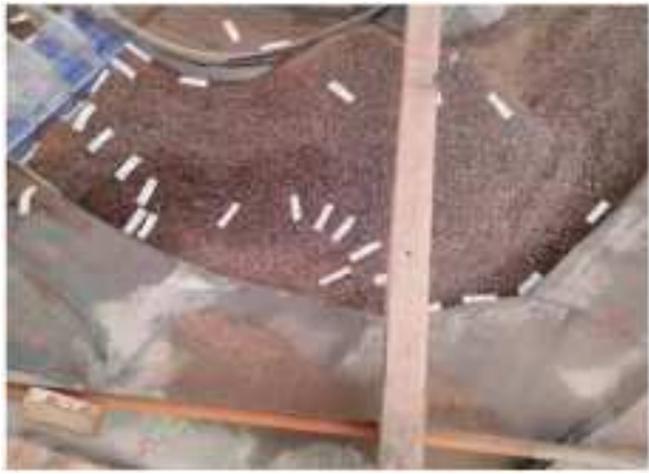
图 2 原方案 200 a 一遇洪水频率下下游河床冲刷情况 Fig. 2 The erosion of downstream riverbed in the original scheme at 200-year flood frequency
