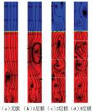
图 10 试验井水位下降状态气液两相分布和流线图 Fig. 10 Gas-liquid two-phase distribution and streamline diagram of test well water level declining state
