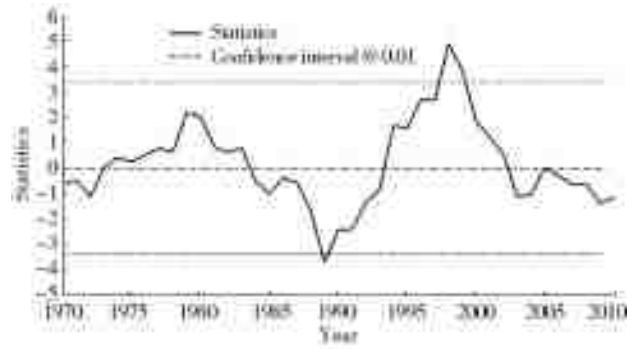
Fig. 4 Variation of moving t -test for interannual runoff at the research area
